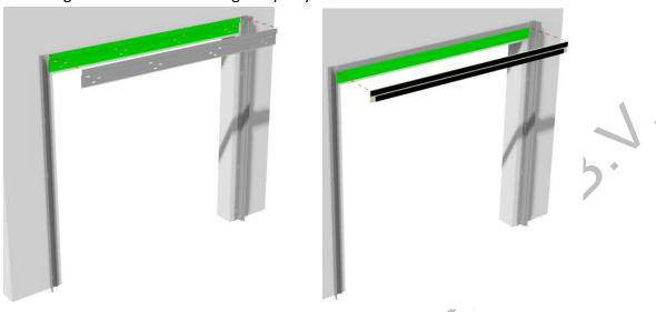
Step 2 B: Mounting the vertical seals on the flame hook profile
