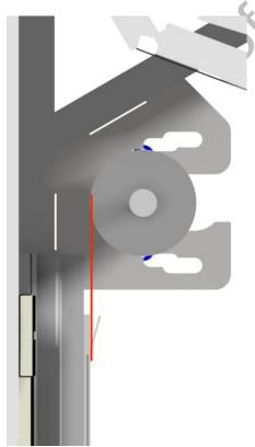
The tangent plane of the pressure roller must be in line with the front of the guide; it must not be positioned closer to the wall.
